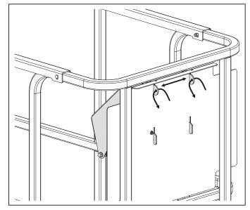
Figure 4-2. Securing Control Station to Platform
