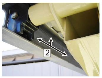
Figure 6-3. Upper Slide Pad Channel
