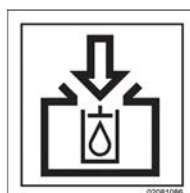
Hydraulic oil reservoir inlet
