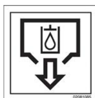
Hydraulic oil reservoir outlet
