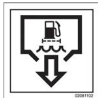
Water sump fuel filter outlet
