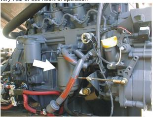
B. Fuel Filter - Deutz TD2.9 (On Engine) Lube Point(s) - Replaceable Element Interval - Change in accordance with engine manual
