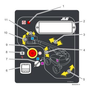
Figure 5. 800S HC3 Ground Control Station
