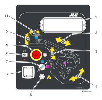
Figure 6. 800S HC3 with MSSO Ground Control Station
