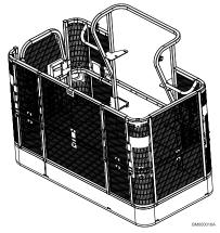
Figure 39. Platform Mesh to Mid Rail
