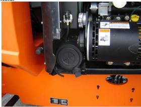
Fuel Filter (Propane) - Ford 2.5L Engine Interval - 3 Months or 150 hours of operation Comments - Replace filter. Refer to Section — Propane Fuel Filter Replacement, Propane Fuel Filter Replacement
