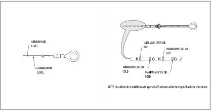
Figure 52. Deutz 2011 Engine Dipstick
