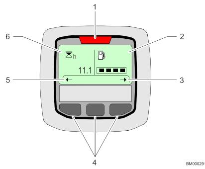
Figure 14. Ground Control Console Display Gauge
