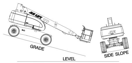
Figure 23. Grade and Side Slope
