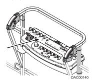
Operator passes through path of sensor beam.
