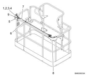
Figure 34. Bolt-On External Fall Arrest System
