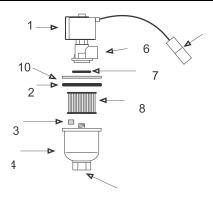
Figure 53. Filter Lock Assembly
