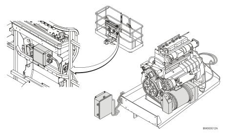
Figure 47. SkyPower and Generator Systems
