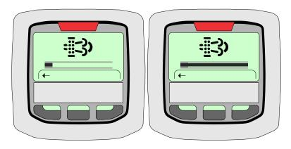
After the cleaning process is complete, the engine will run for approximately 5 minutes to allow the engine and Exhaust After Treatment (EAT) to cool down. The Indicator Gauge will display the "Regen Complete" screen as shown and the Emissions Temperature indicator will no longer be illuminated.
