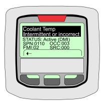
Figure 13. Engine Diagnostic Screen
