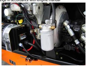
C. Fuel Filter - Deutz TD2.9 (On Hydraulic Tank) Lube Point(s) - Replaceable Element Interval - Change in accordance with engine manual
