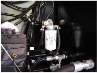
D. Fuel Filter - China III Lube Point(s) - Replaceable Element Interval - Every year or 600 hours of operation
