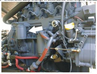
B. Oil Change with Filter - Deutz TD2.9 Lube Point(s) - Fill Cap/Spin-on Element Capacity - 9.6 Quarts (9.0 L) Lube - EO Interval - Every Year or 600 hours of operation Comments - Check level daily/Change in accordance with engine manual.
