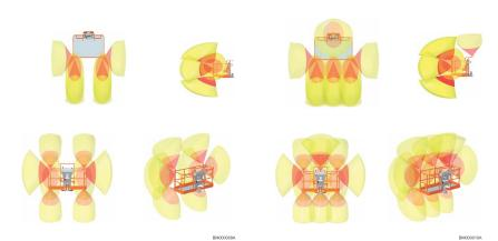
Figure 48. SkySense Coverage Level 1 Areas (2– Bar)
