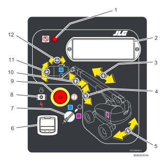
Figure 8. 860SJ HC3 Ground Control Station
