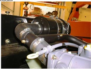
B. Air Filter (Deutz TD 2.9) Lube Point(s) - Replaceable Element
