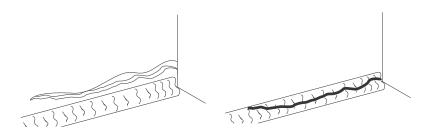
Figure 2. Parent Metal Crack
