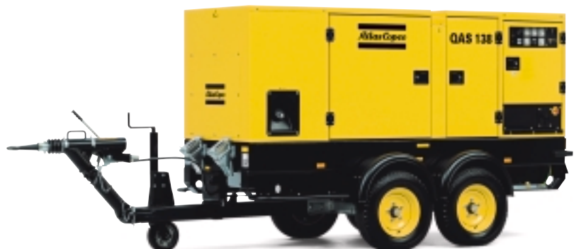
Twin axle portable generator
